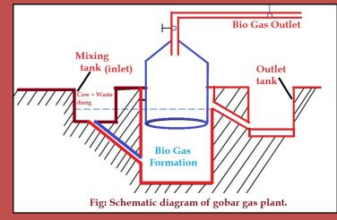
Slurry of cow dung and other waste is added in mixing tank. This slurry is then sent to digester tank where slurry is allowed to get decompose for 10/15 days and then produces gases like methane, hydrogen sulphide and  $CO_2$ . The bio gas is stored in a tank mounted above digester tank and can be used via outlet provided with tap.
